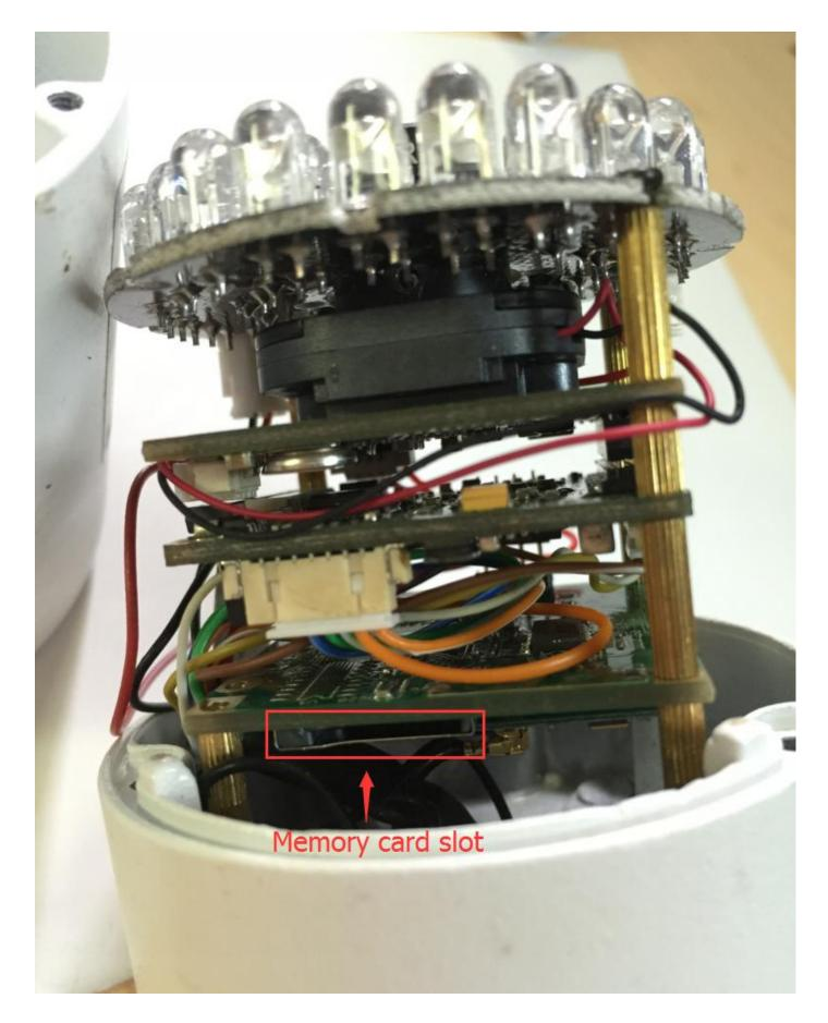
3. Insert SD card into the slot, when hear "click", it means succeed. (press the SD again, the SD card will eject)
