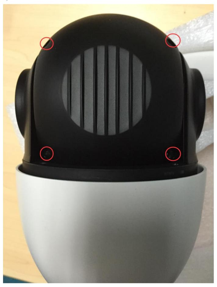
2. Take off camera back cover, disassemble 2 screws as picture shown.
