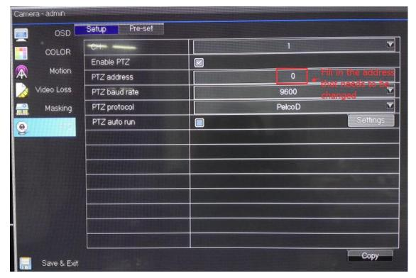
3, In PTZ control section, call 80 preset to open camera address.
