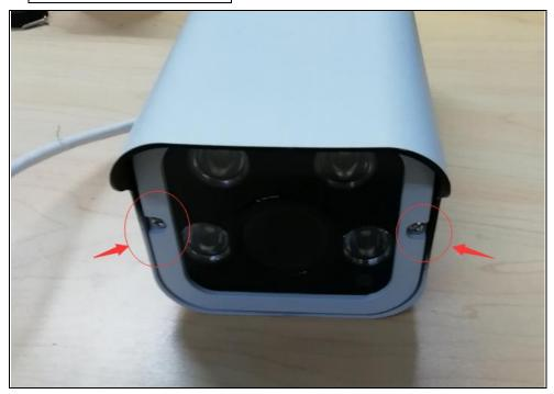
2.the SD card slot is located in the place with red arrow
