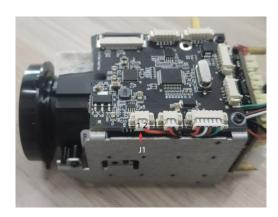
Remarks: This movement supports VISCA protocol (connected to Speed dome PTZ camera) and PTZ serial port protocol (connected to PTZ). The default is VISCA protocol.
